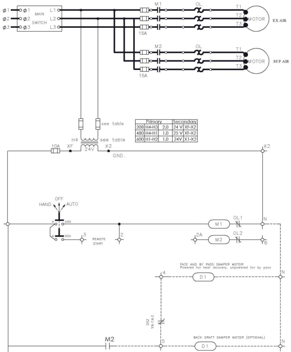
Use auxiliary contacts M1 and/or M2 to interlock with other equipment. M1 and M2 are N.O., dry and close when the motor is operating. Field wiring is done at the contact block, i.e. terminals not provided.
