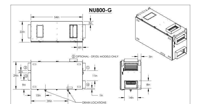
3 - RETURN AIR / EXHAUST AIR FROM SPACE 4 - EXHAUST AIR / EXHAUST AIR TO OUTSIDE
