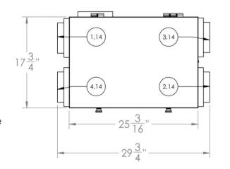
Unit is Reversible 2 Doors are removable if required for access to core and routine maintenance
