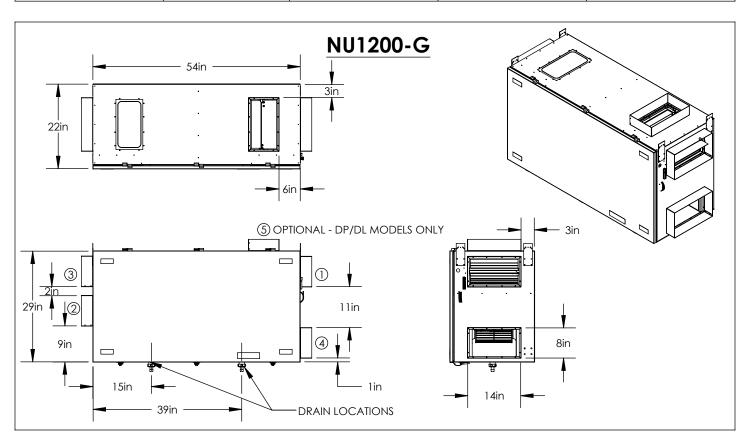
3 - RETURN AIR / EXHAUST AIR FROM SPACE 4 - EXHAUST AIR / EXHAUST AIR TO OUTSIDE 5 - DEFROST AIR (OPTIONAL - DP/DL MODELS ONLY)
