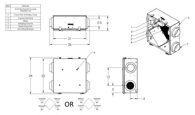
The airflow configuration is reversible out of the box without any installer intervention.
